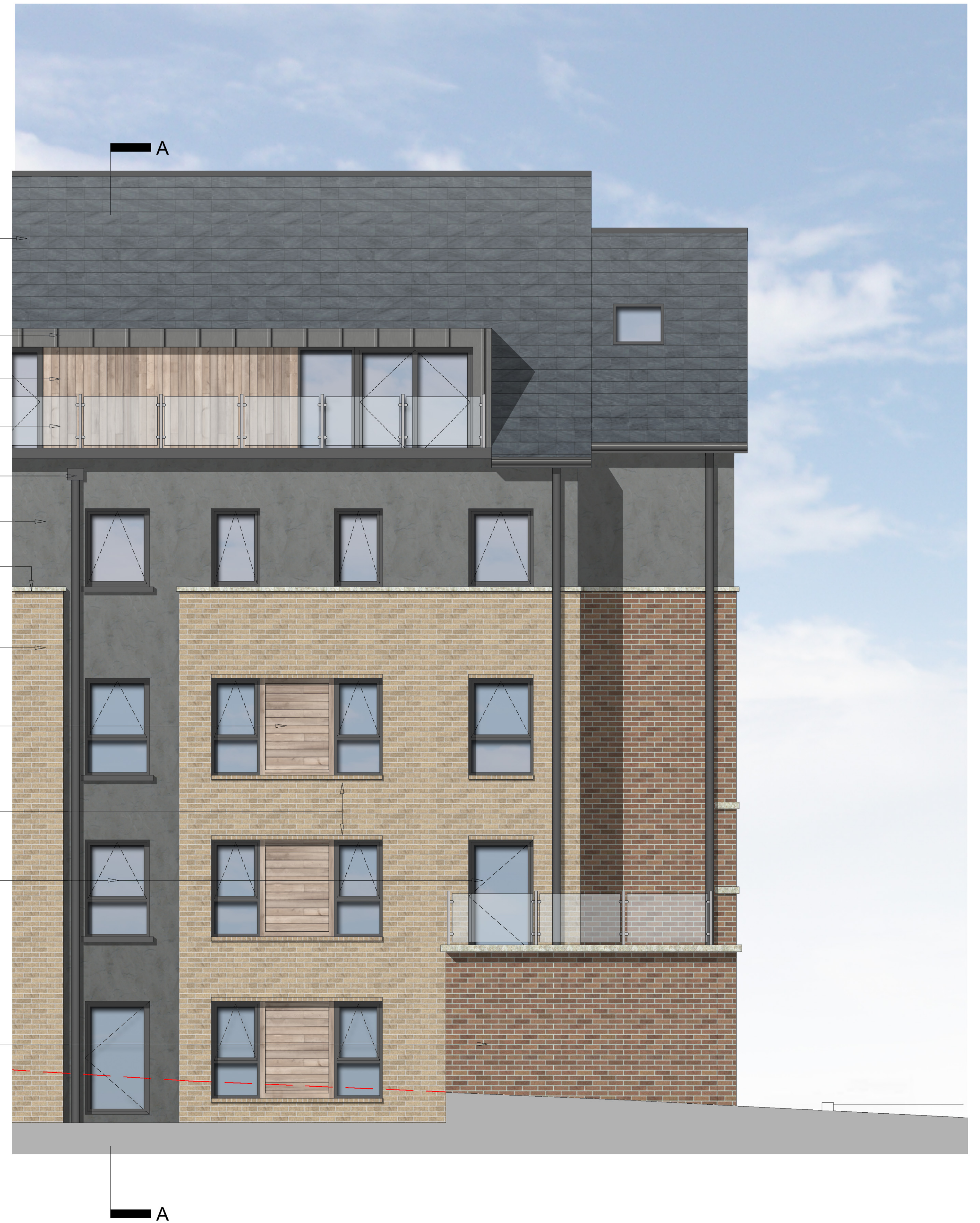
Bay Elevation showing indicative proposed materials 1 : 50
